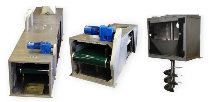
Continuous weighing line for fiberized cellulose
