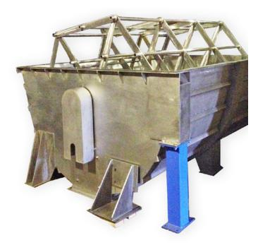
On the line of continuous weight dosing, the fiber cellulose is supplied from an intermediate hopper-agitator.
