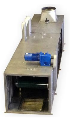
The loading conveyor has viewing windows for the possibility of observing the process of loading cellulose into the prednitrator.
